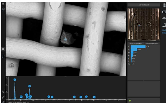
Live EDS analysis of particles inside metal mesh.
